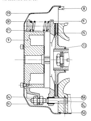
For a two brake disc FCPL, the disc the nearest to the armature 11 must be mounted without O-Ring seal 73.
